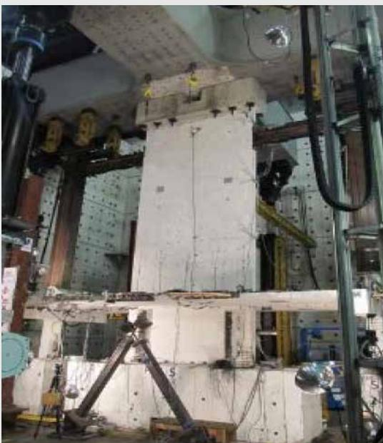
Unbonded Post-Tensioned Rocking Wall Specimen
