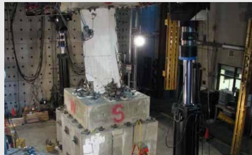
Large Scale Reinforced Concrete Column
